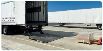
This is what a liftgate looks like when it's fully deployed. This model is a tuck-under liftgate.
