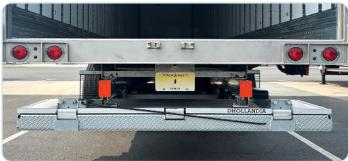
There are two main types of liftgates: rail-style liftgates, which are mounted directly to the rear of the truck, and tuck-under liftgates, which fold and store beneath the truck when not in use.
