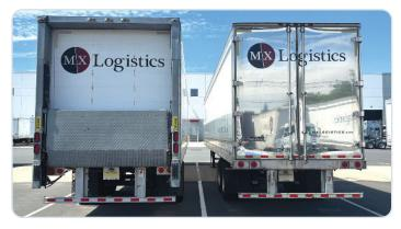
There are two main types of liftgates: rail-style liftgates, which are mounted directly to the rear of the truck, and tuck-under liftgates, which fold and store beneath the truck when not in use.
